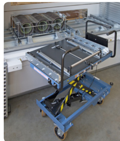
Tray with transfer station and transport trolley for grinding wheels
