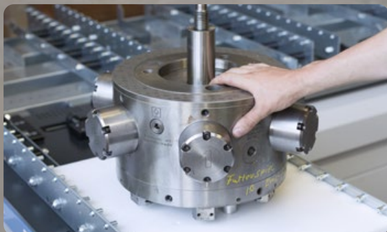
Tray with transfer station and transport trolley for extremely heavy, shock-sensitive lathe chucks in the plant of an automobile manufacturer
