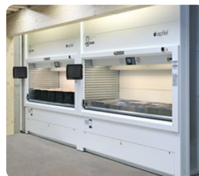
Tandem tool towers in ESD design with access openings on two floors
