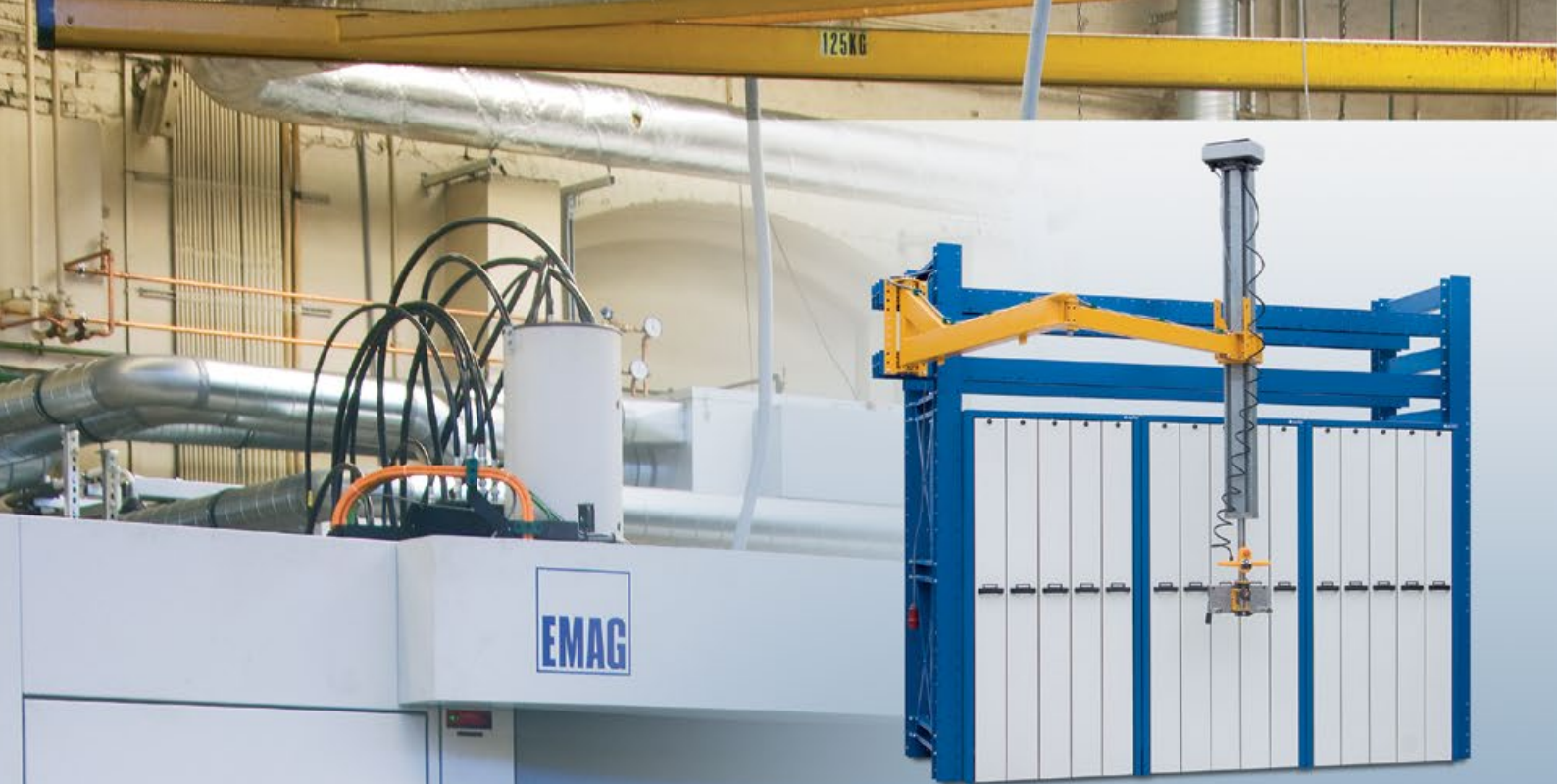
Storage system for broaches with swivelling lifting device
