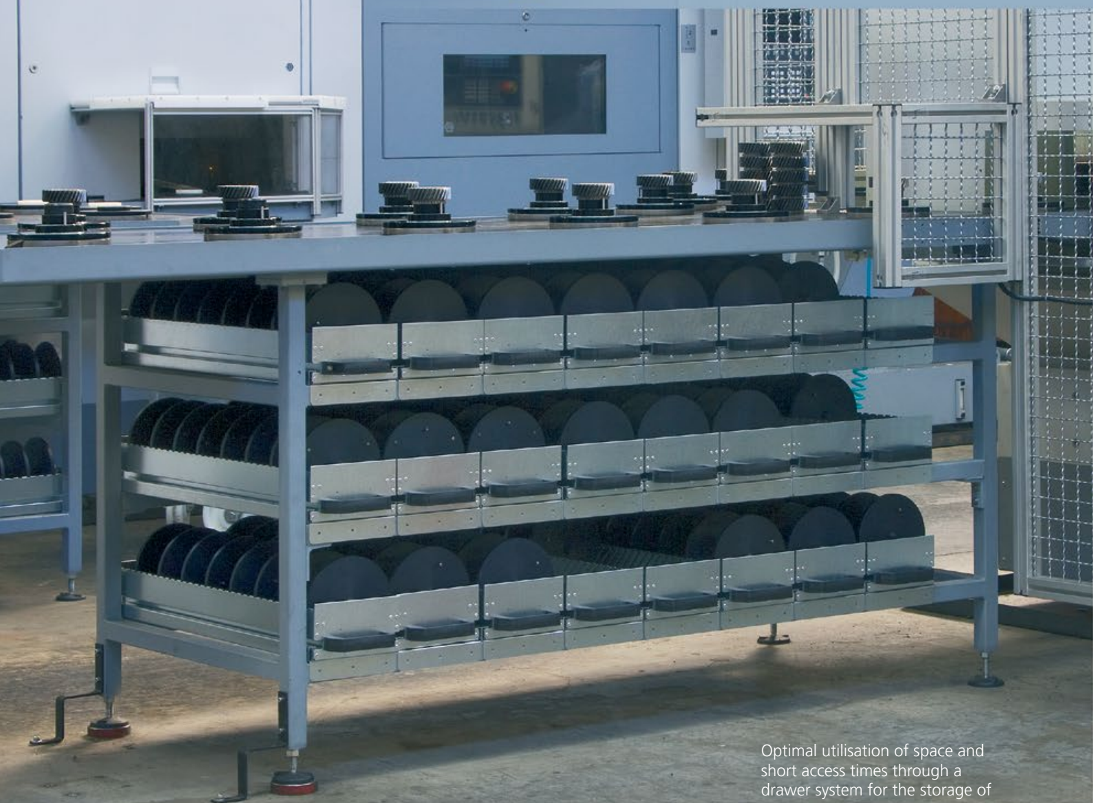
Storage system for broaches with swivelling lifting device
